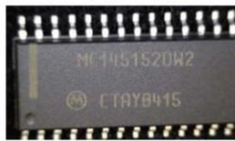
**All of them are counterfeit! All of the top surfaces you see have been altered to mislead the buyer into thinking the parts are authentic. All of the parts should be considered unreliable.**
