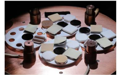
Samples of thermal control materials under test in the VADAR Facility
