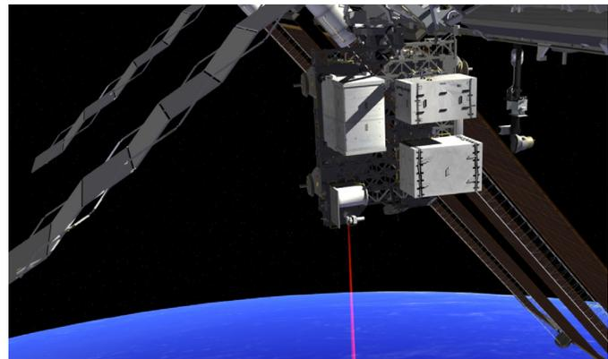
Optical Payload for Lasercomm Science (OPALS) was developed at JPL and tested on the ISS in 2014 to demonstrate laser communications between spacecraft and ground stations. Credit: NASA.
