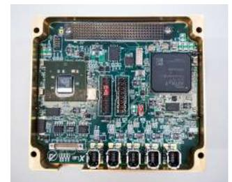
Handle, Slingshot’s payload electrical interface module.
