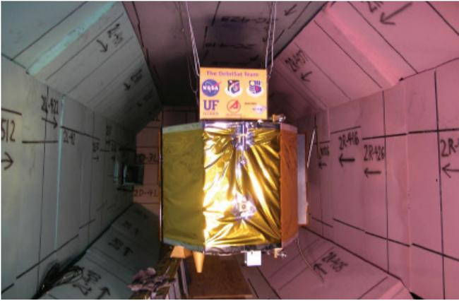
DebrisSat before and after the collision. The DebrisLV test was conducted on April 1, 2014, followed by the DebrisSat test on April 15. Both tests used an aluminum and nylon cylindrical projectile with a mass of slightly less than 600 grams and propelled
