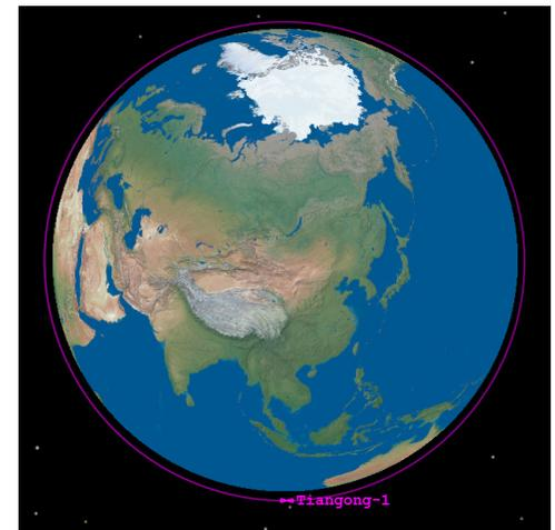
Orbit of Tiangong-1 as of March 13, 2018 @ 00:00:00.000 UTC. The apogee (highest point in the orbit) = 259 km, while the perigee (lowest point in the orbit) = 231 km. For reference, the International Space Station is in a 400 km circular orbit.
